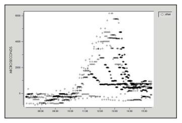
Figure 1: NTP offset vs. NTP server (Thesys) vs. time of day, 10 days of data
