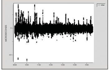
Figure 2: TimeKeeper offset vs. Time server (Thesys) vs. time of day, 14 days of data
