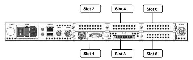
Figure 1: NetClock 9483 rear panel option module bay slots
