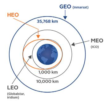
Space orbits are an important consideration when testing space missions due to their unique characteristics. Of equal concern is the high number of satellites visible, and high signal power variations (signals from outside boresight).
